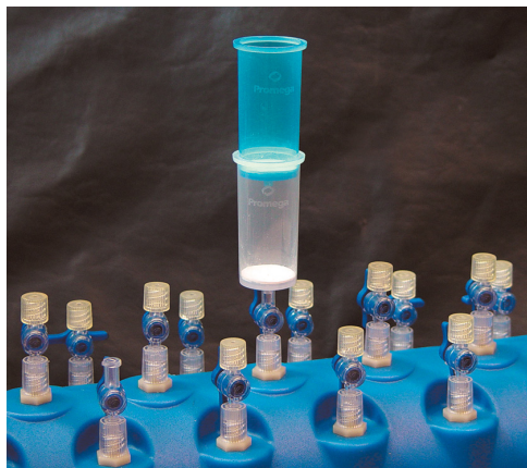
Figure 1. The blue clearing column inserted into the white binding column. The two columns sit on a vacuum manifold port.
