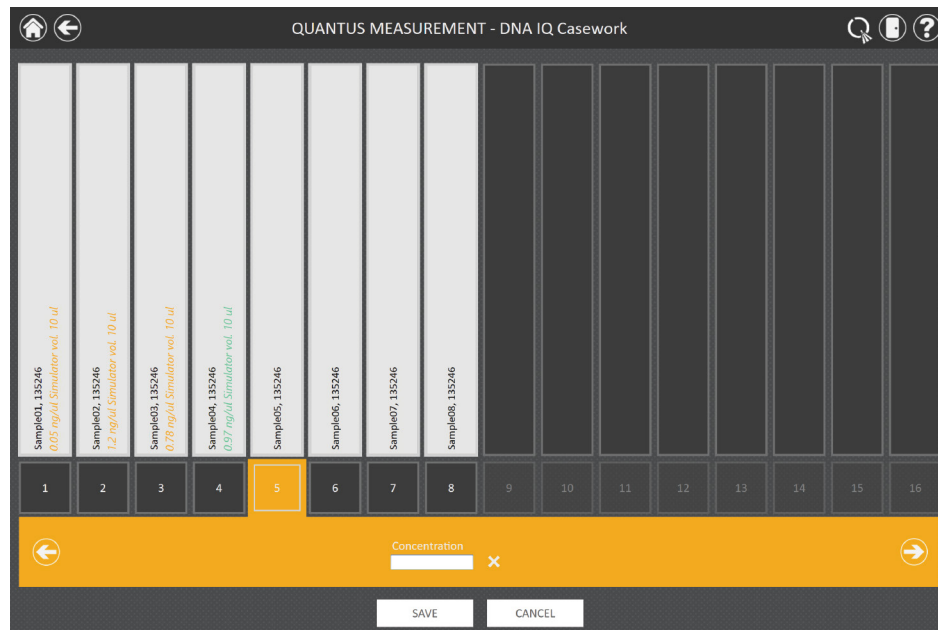
Figure 56. 'Quantus Measurement' screen. After making a quantitation measurement with the Quantus™ Fluorometer, the quantitation value is displayed to the right of the sample identifier.
