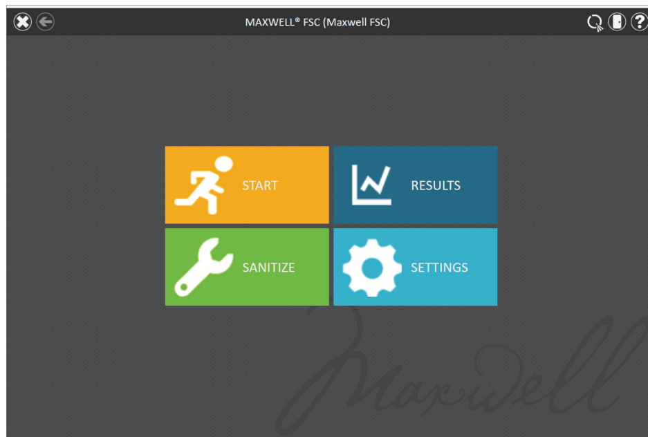
Figure 65. 'Home' screen. Selecting the Sanitize button begins the process for UV treatment of the Maxwell® FSC Instrument.
