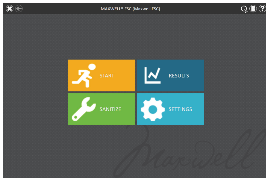
Figure 53. Maxwell® FSC 'Home' screen. When the Quantus™ Fluorometer is correctly connected to the Maxwell® FSC, the “Q” logo is displayed in the upper right corner of the title bar.
