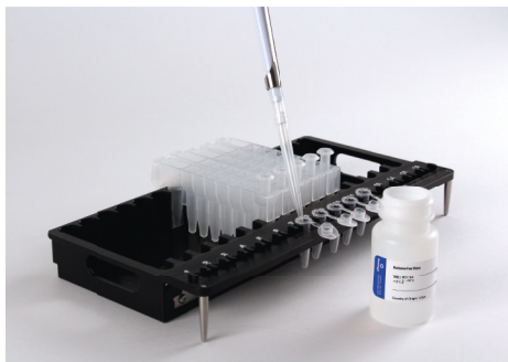
Figure 3. Setup and configuration of the deck tray(s). Elution Buffer is added to the elution tubes as shown. Plungers are in well #8 of the cartridge.
