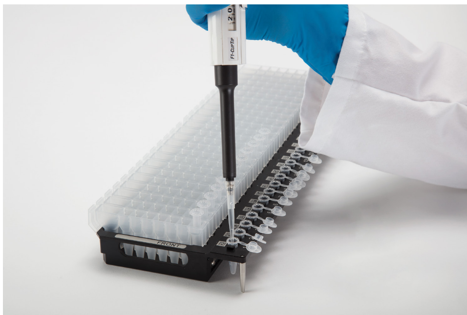
Figure 2. Setup and configuration of the deck tray. Maxwell® DE elution mix is added to the elution tubes as shown. Plungers are in well #8 of the cartridge.
