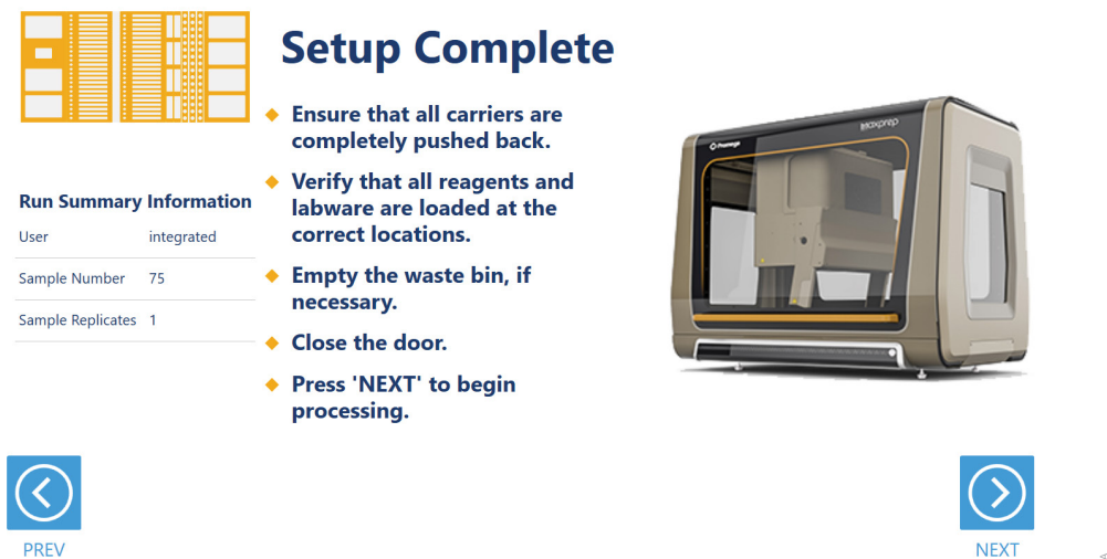
Figure 23. Final instrument setup screen. This screen presents a list of items that should be checked before starting automated processing. It also provides a final chance to return to any of the previous instrument setup screens before automated processing begins. To start processing, close the instrument door and press the Next button.
