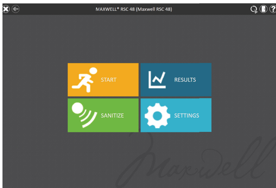
Figure 33. Maxwell® RSC 48 'Home' screen. Selecting the Start button begins the process of running an extraction method on the Maxwell® RSC 48 Instrument.
