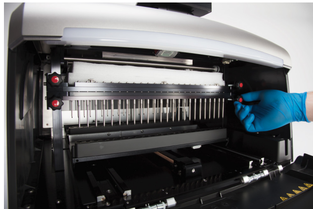
Figure 69. Placement of plastic stoppers. Move the magnet and plunger bars up, and secure the four shipping screws on both sides of the magnet and plunger bars.
