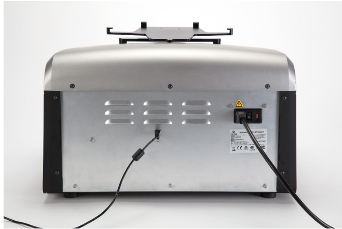
Figure 10. Connecting the Tablet PC to the back of the Maxwell® RSC 48 Instrument.
