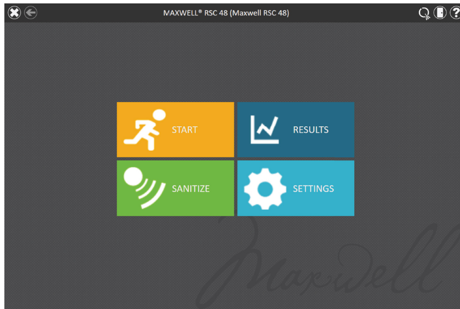
Figure 63. 'Home' screen. Selecting the Sanitize button begins the process for UV treatment of the Maxwell® RSC 48 Instrument.
