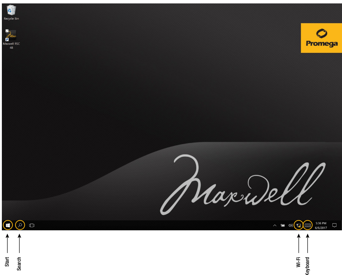
Figure 74. The 'Desktop' Screen. At the bottom of the 'Desktop' screen is the task bar. Access to the options and settings referenced in this document is provided by the Windows® Start, Search, Speaker, Wi-Fi and Keyboard buttons in the task bar.
