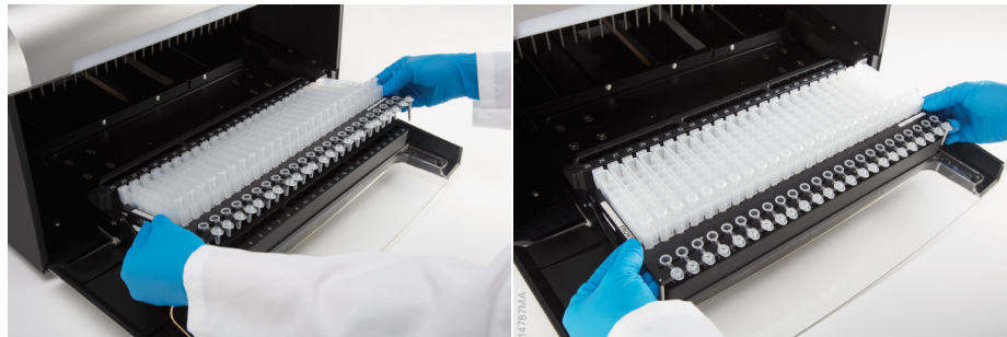
Figure 43. Placing the deck tray in the instrument.
