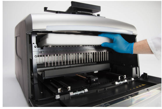
Figure 8. Removing the top foam from the instrument. Move the magnet and plunger bars downward to remove the top foam piece.
