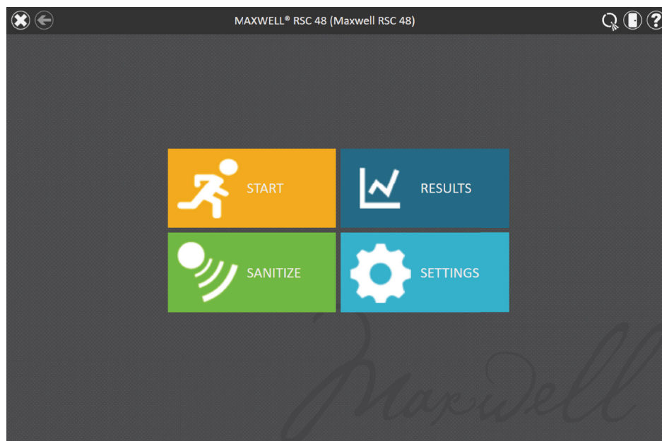
Figure 51. Maxwell® RSC 48 'Home' screen. When the Quantus™ Fluorometer is correctly connected to the Maxwell® RSC 48, the “Q” logo is displayed in the upper right corner of the title bar. Prior to quantification, verify the Quantus™ Fluorometer has the appropriate protocol selected. If the Quantus™ Fluorometer needs calibration or the mode needs to be changed, consult the Quantus™ Fluorometer Operating Manual #TM396 .
