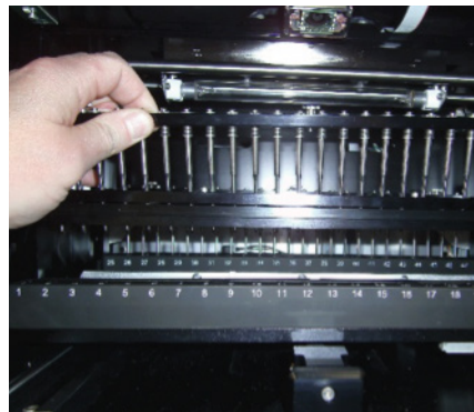
Figure 66. Removing the front magnetic rod assembly. Panel A. Loosen the three thumbscrews that hold the magnetic rod assembly on the magnet bar. Panel B. Move the deck forward and slide the magnet bar down. Slide the magnetic rod assembly up and forward to remove it from the magnet bar.
