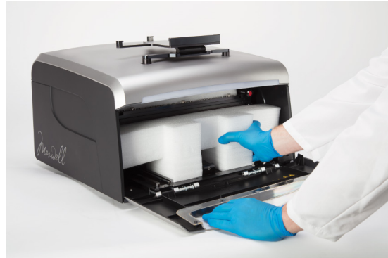
Figure 70. Insert the front die-cut foam. Make sure the serrated edge covers the magnet rods.
