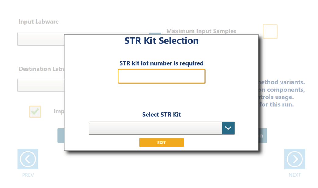
Figure 4. Providing Promega STR kit information. An initial pop-up screen requests information regarding the lot number for the Promega STR kit being used for this run and a drop-down menu for selection of the specific kit to be used.
