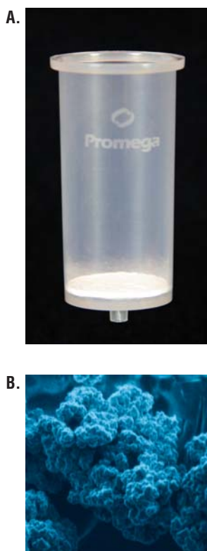
Figure 9.1. Images of two Promega silica purification matrices. Panel A. A PureYield™ Midiprep binding column. The membrane is present at the bottom of the column. Panel B. An electron micrograph of MagneSil® PMPs.
